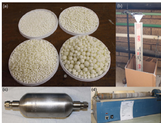
Fig. 24. (a) The pellet with different diameters of Zr-MOF. (b) Set up of drop test for dropping mechanical strength. (c) Cylinder packed with Zr-MOF. (d) Set up of abrasion test for tumbling mechanical strength. Reproduced with permission from [159]. Copyright 2015 Elsevier.
